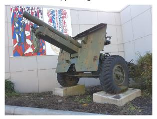
On the 5th August 2017 that was all set to change as a tow truck turned up to take the cannon away. The cannon was dismantled, sand blasted, rust cut out, repairs made and re welded. While this was going on J contacted an historian at ANZAC House who provided him with some of the cannon's history and the colour code.
